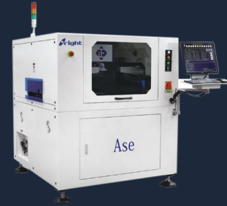
Fully automated solder paste printer
